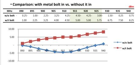
•BLADE reads best without any metal bolt in two holes. With RF interference, metal bolts decreases read range by 40% or more. RFcamp recommends not using metal bolts, but 3M 300LSE adhesive or glue for maintaining optimum read performance. In case adhesive or glue can not be used, polycarbonate (or nylon) bolts is recommended.
