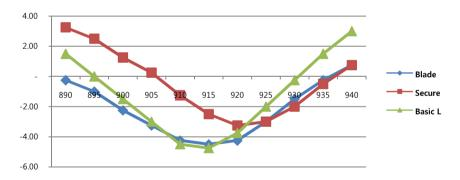
•BLADE reads up to 6.5 meters on metal, 20% longer than SECURE and 10% shorter than FASTENER. Its read performance is best among similar slim size metal tags with such low profile of 4mm thickness.
